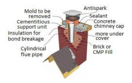
Smoke chimneys should not be placed on the outer wall of the building unless there is a technical necessity. The wall thickness of the chimney walls should not be less than the thickness of one brick. Perforated bricks and briquettes should never be used in chimney construction. It should be plastered from the inside and outside and a
